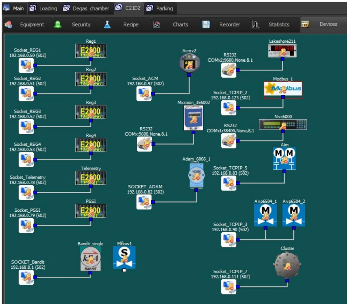
The *Devices* tab is a visual representation of the chamber electronic devices that can communicate with *Crystal XE* and allows you to easily detect a communication or a connection problem.
