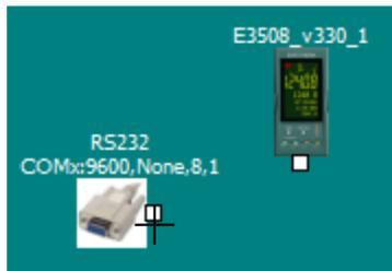
Then drag the cursor between the port and the device in order to create a link.
